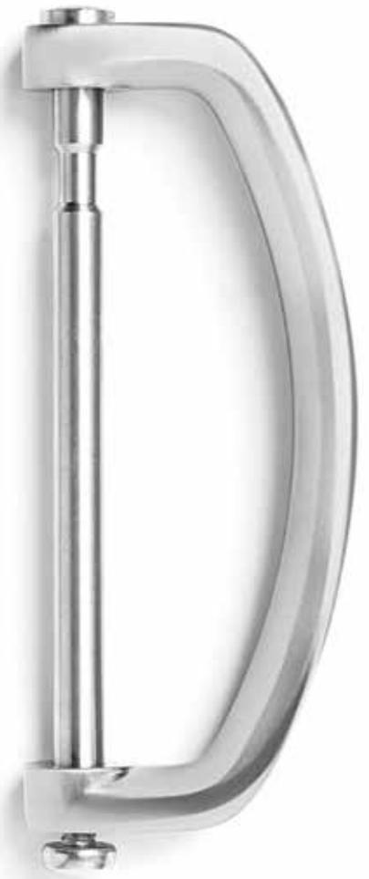
The secondary and D-handle – both of which have been specifically designed by Origin to withstand a pull of 1600 Newtons – are available in any one of the 150 RAL shades or a stainless steel finish, so they can be matched or contrasted to the door itself.
