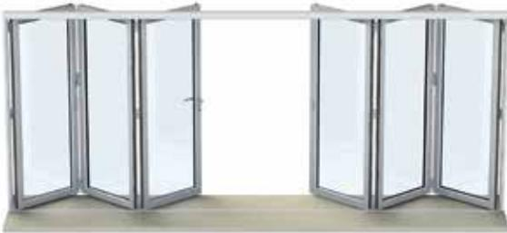
Ideal for larger openings, the 3+3 is one of the most diverse configurations as it can operate as a French door at the center, have 3 doors opening one way while the other 3 remain closed, or they can be opened fully with 3 doors folding each way to offer complete symmetry.
